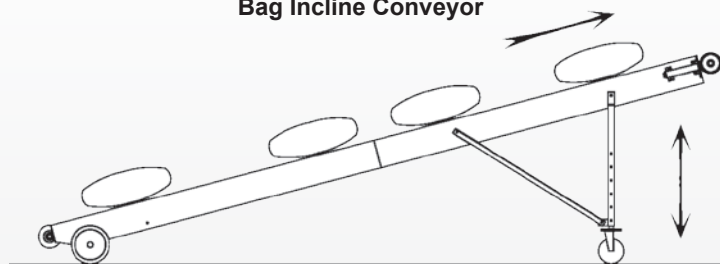
Bag Incline Conveyor
