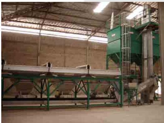
3 hopper Weighcont Blender + Small bag Filling Machine
